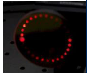
Typical Herriott cell spot pattern
